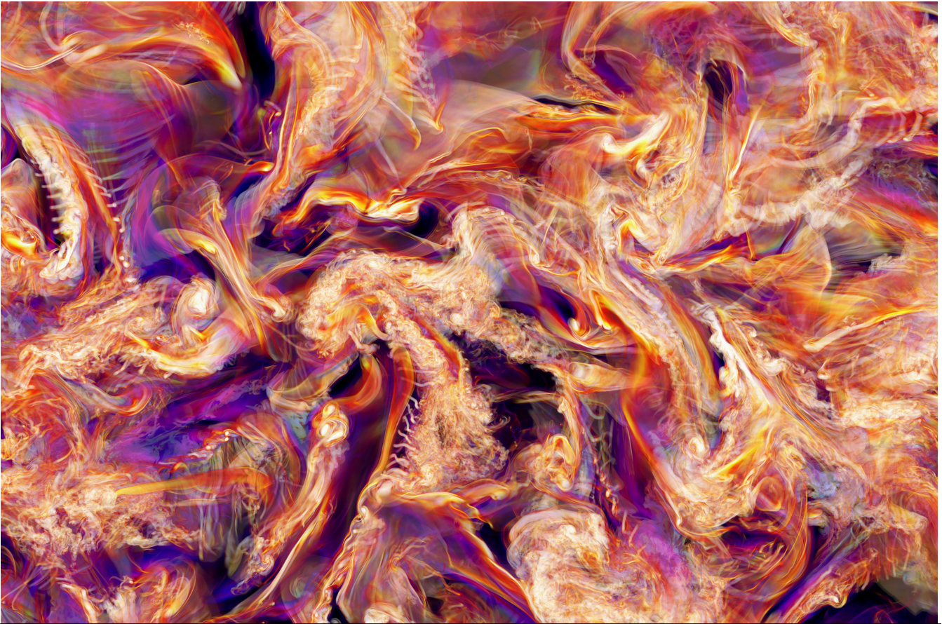
Fig. 1D. Volume visualization of the distribution of the magnitude of the vorticity in a thin slice of the PPM simulation of Mach 1 homogeneous turbulence discussed in the text. The relation between color and vorticity magnitude is identical to that in Fig 1b. Here the flow is shown at the time of Fig 1b, viewed closer up but from the same angle and with clipping planes making only a slice of the domain near the center visible. The slice shown extends across the entire diagonal width of the cubical problem domain, revealing the wealth of detail that is captured by the PPM scheme operating on this very fine, 2048^3 grid. This high degree of captured detail allows predictions of alternative turbulence closure models to be compared with the simulation data to generate statistically significant quantitative measures of their predictive capability.
