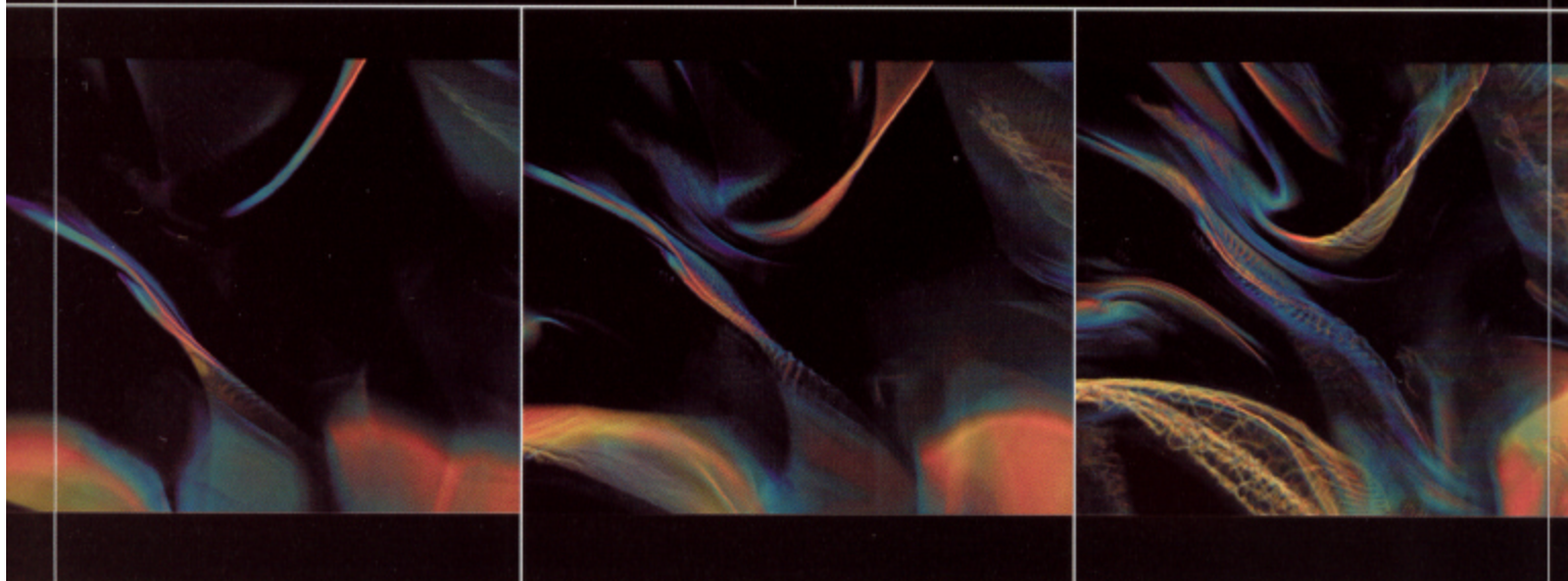
Vorticity at three intervals in a turbulent flow. Blue and cyan indicate low vorticity, orange shows mid-level vorticity, and yellow indicates high vorticity. Over time the turbulent flow shows more vorticity.
