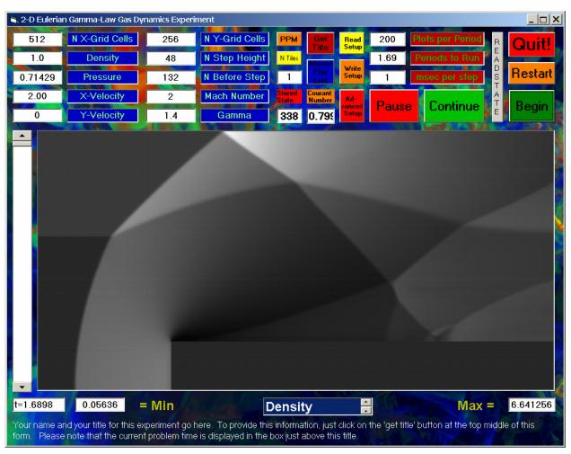
location of the bow shock, the air slams into the compressed air that has piled up in front of this obstacle. The shape of this bow shock, swept back as we get further away from the step in the vertical direction, is not unfamiliar. It is, after all, not that different from the shape of the bow wave set up by a boat moving through the water of a lake.
