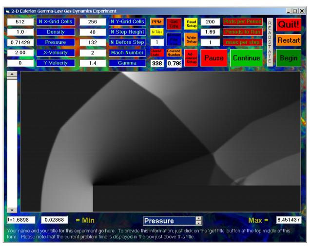
shown on the next page, clearly indicates that the gas flowing along the top surface of the step is very hot. This hot gas appears directly after the flow turns around the corner of the step, and it is then transported downstream along the top of the step. Shocks which strike the top of the step must interact with this thin layer of hot gas, and one of these interactions led to the formation of the small recirculation region revealed in the x-velocity plot.
